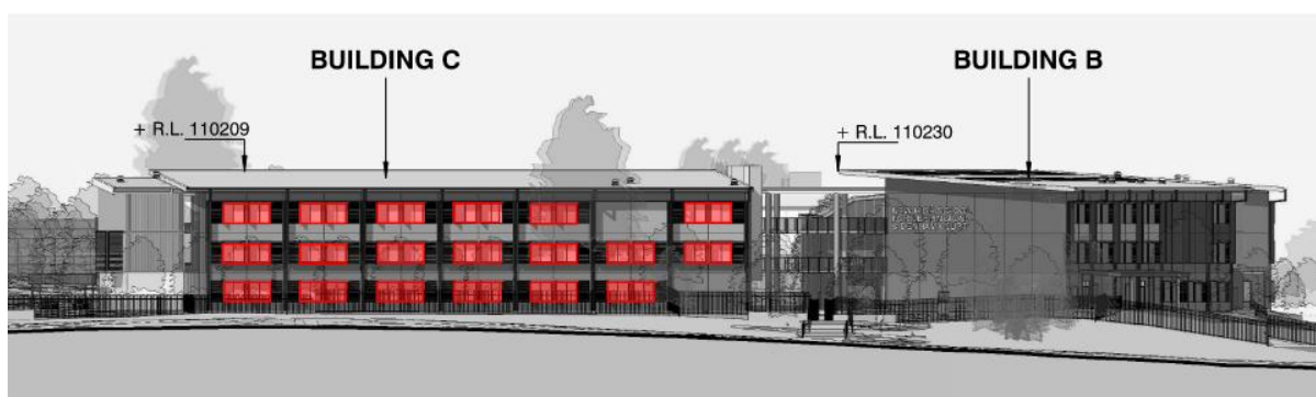
Figure 9: External glazing recommended to achieve a minimum sound reduction index of R_w + C_{tr}33 (red highlight).
