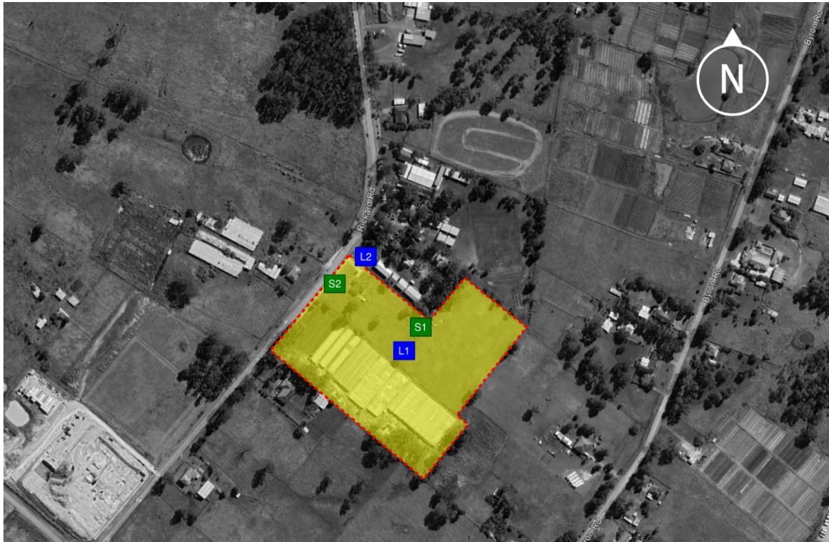
Figure 4: Noise survey locations and boundary of the site. (Long-term monitoring - L1, Long-term monitoring conducted for Leppington Primary school – L2, short-term monitoring S1 & S2).
